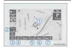
To scroll over the map screen, place the cursor mark in the desired position and then press and hold the Remote Touch knob.
