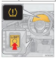
Press and hold the tire pressure warning reset switch until the tire pressure warning light blinks slowly 3 times.
