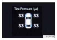
The tire pressure detected by the tire pressure warning system can be displayed on the multi-information display.  $(\rightarrow P.28)$
