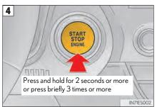
To stop the engine, press and hold the engine switch for 2 consecutive seconds or more, or press it briefly 3 times or more in succession.
