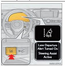
Press the LDA switch to turn the LDA system on.
