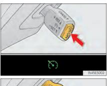
1 Press the "ON/OFF" button to activate the cruise control.
